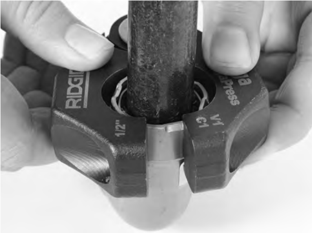
Figure 11 – Installing Press Ring Onto Fitting
