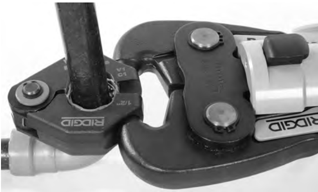
Figure 12 – Attaching Actuator to Press Ring
