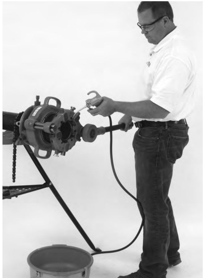
Figure 7 – D-1440 Ratchet Operation
