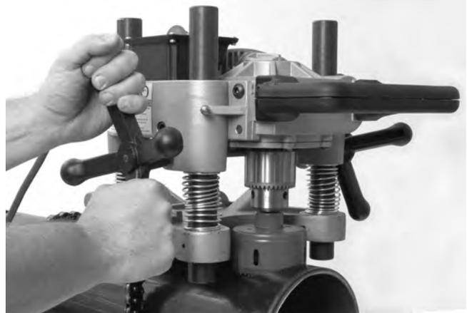
Figure 11 – Operating the Hole Cutting Tool
