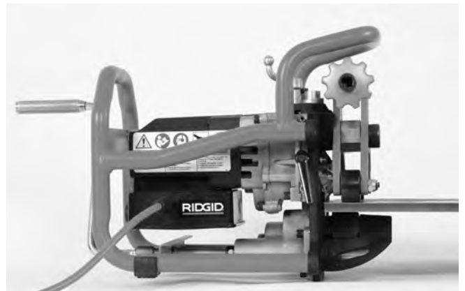
Figure 16B – Installing Beveller on Plate
