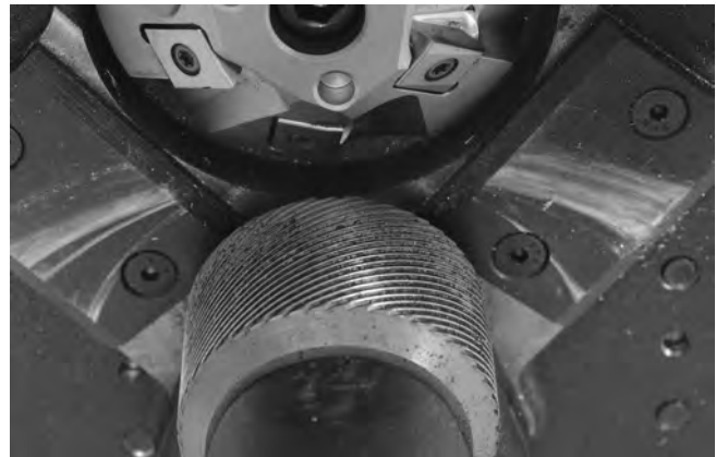
Figure 22– Clean Drive Roll Knurls
