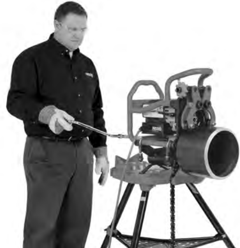
Figure 20C – Bevelling Operation (Fixed Beveller/Rotating Pipe)
