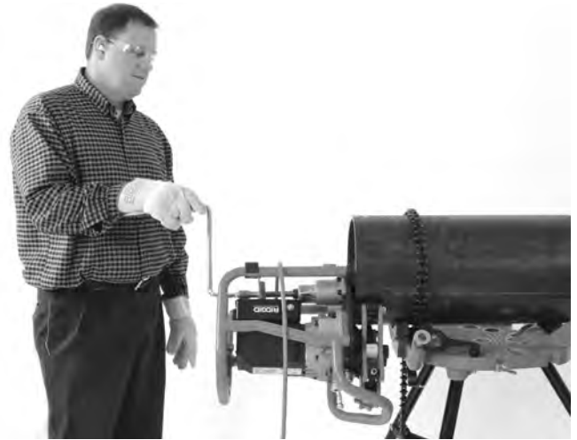
Figure 20B – Bevelling Operation (Fixed Workpiece/Moving Beveller)
