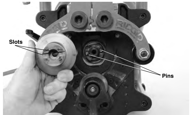
Figure 25B – Replacing Cutter Heads
