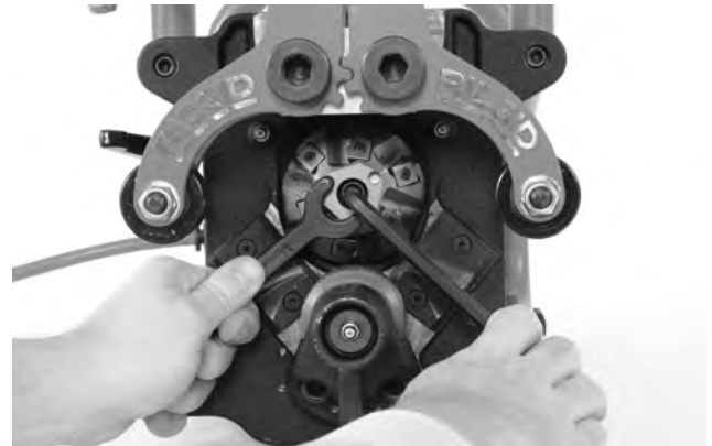
Figure 25A – Changing Cutter Heads
