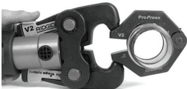
Figure 10 – Attaching Actuator To Press Ring
