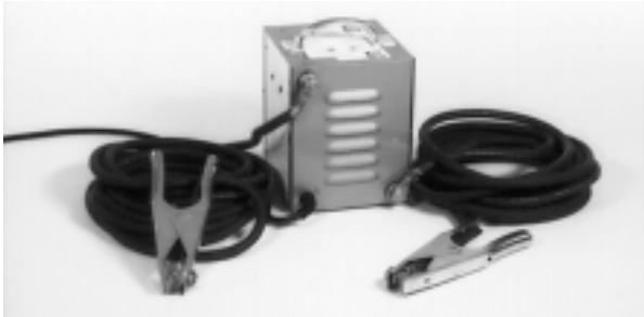
Figure 3 – Thawing Tool with Cables Installed
