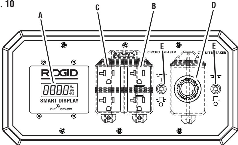
A - SMART DISPLAY monitoring system (système de surveillance SMART DISPLAY, sistema de monitoreo SMART DISPLAY)
