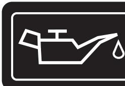
Add lubricant to full mark to start. Engine will not start or will shut off if sensor detects low lubricant level.
