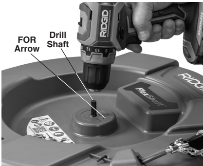
Figure 4 – Attaching Drill To Drill Shaft
