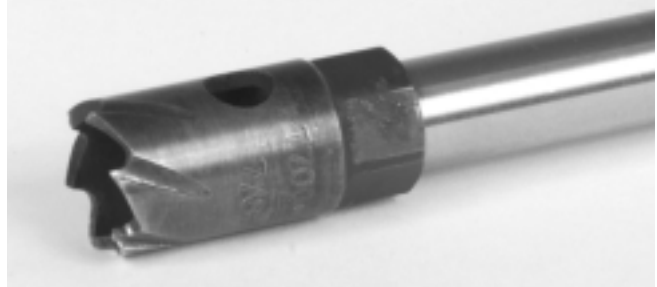
Figure 4 – Installation of cutter on small hole saw arbor
