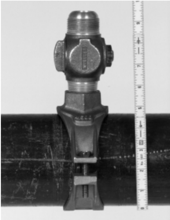
Figure 10 – Measuring maximum stroke
