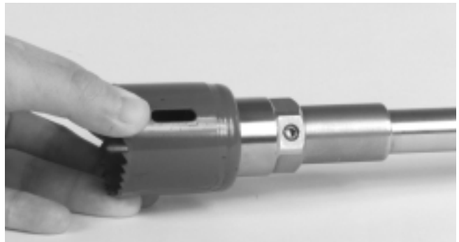
Figure 3a – Installation of large hole saw adapter
