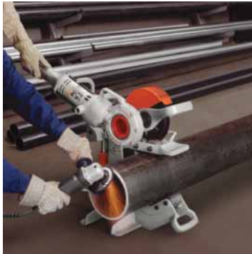
Use Model 258 with the Pipe Roller to rotate pipe when beveling. Two operators are recommend for this operation.
