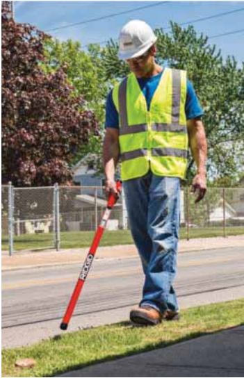
Precisely locate curb stops and other underground objects containing iron.
