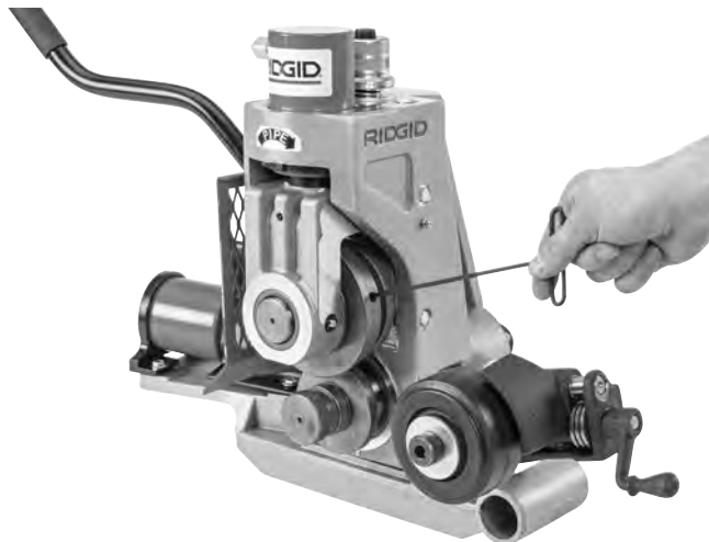
Figure 24 – Loosening Grooving Roll Set Screw
