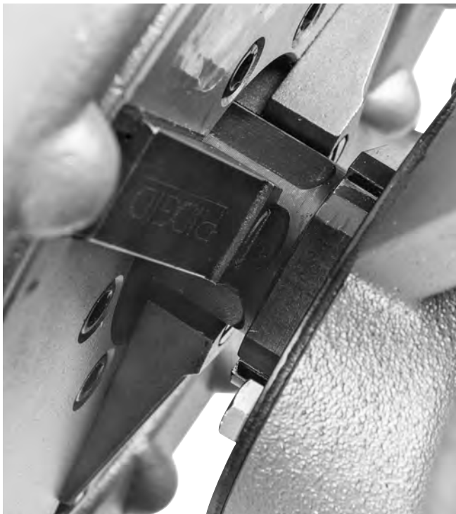
Figure 7B – Securing Drive Shaft In Chuck
