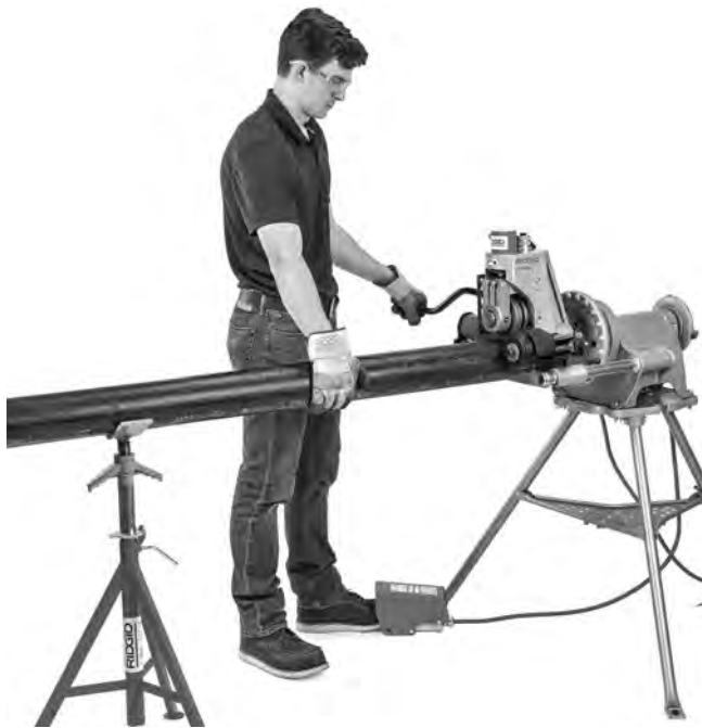
Figure 19 – Applying Pressure on Pipe with Power Drive in REV direction
