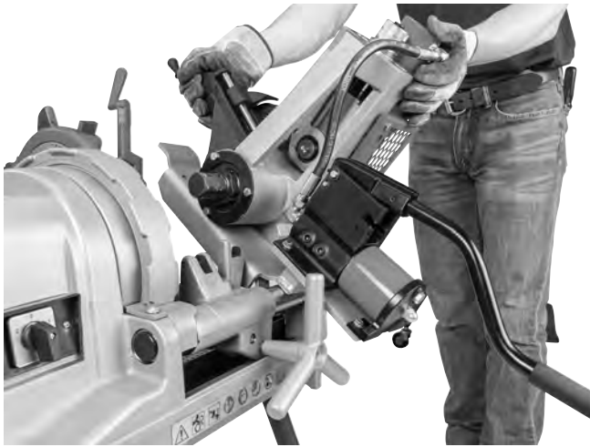
Figure 8B – Installing 918 on 1233 Threading Machine
