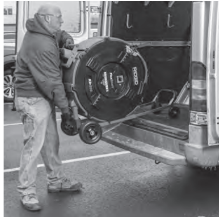
Figure 17 – Lifting Unit Onto Vehicle
