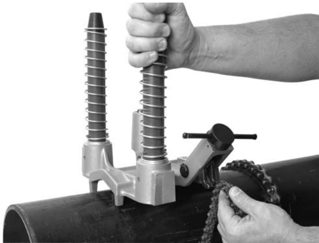
Figure 8 – Hooking the Chain
