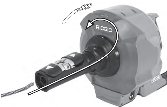
Figure 21 – Loading Cable Without Changing Inner Drum
