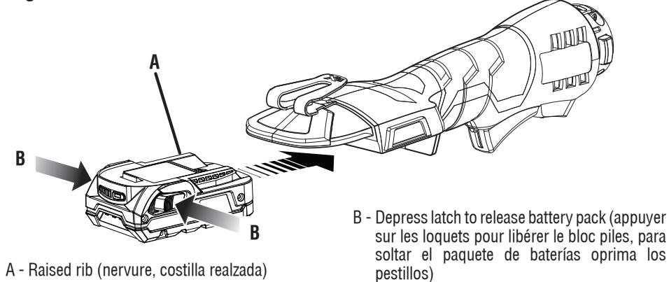
A - Raised rib (nervure, costilla realzada)
