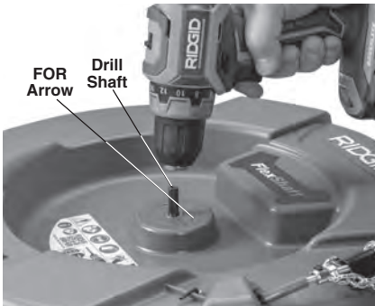
Figure 4 – Attaching Drill To Drill Shaft
