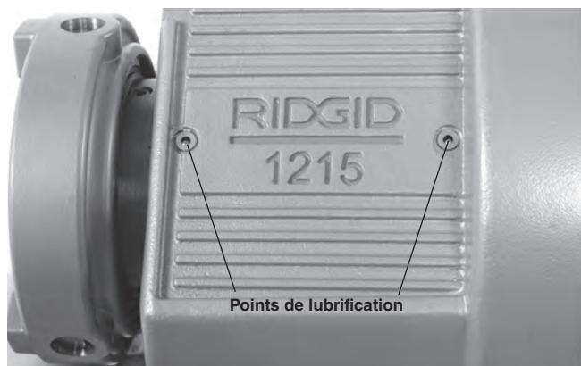
Figure 16 – Points de lubrification
