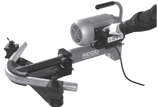
Figure 14 – Operating the Open Wing Bender
