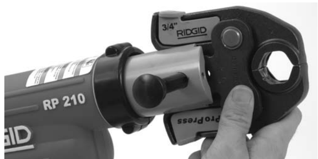
Figure 5 – Slide Attachment Into Tool
