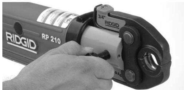
Figure 4 – Fully Open Attachment Mounting Pin
