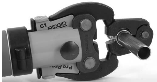
Figure 10 – Attaching Actuator To Press Ring
