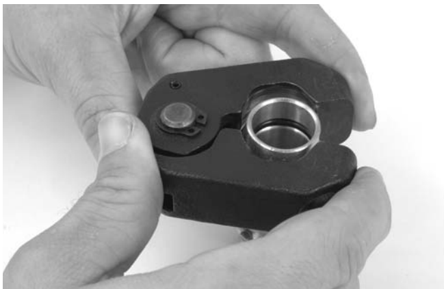
Figure 9 – Installing Press Ring Onto Fitting
