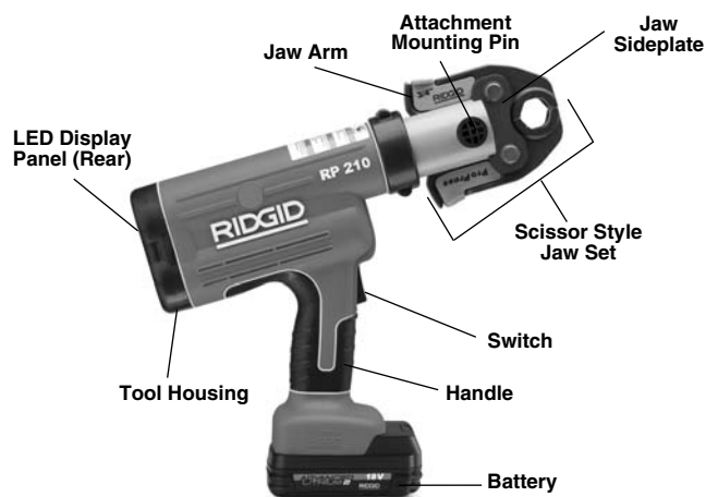
Figure 1 – RP 210-B Press Tool And Compact Series Jaw
