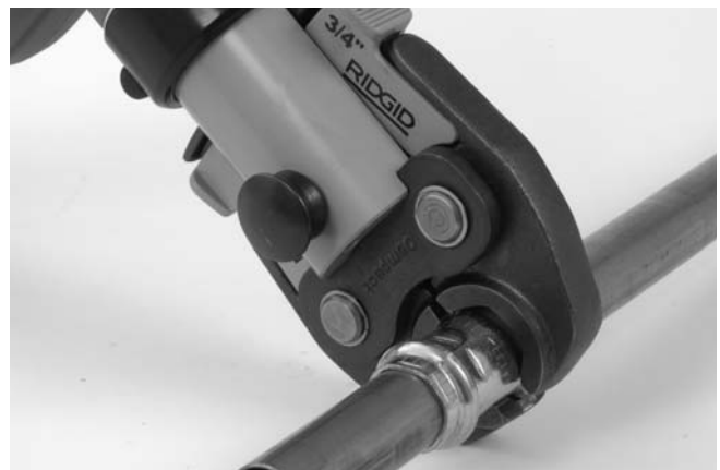
Figure 7 – Placing Scissor-Style Jaw Set Around Fitting
