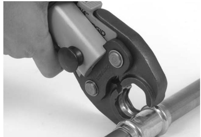
Figure 6 – Opening The Scissor-Style Jaws
