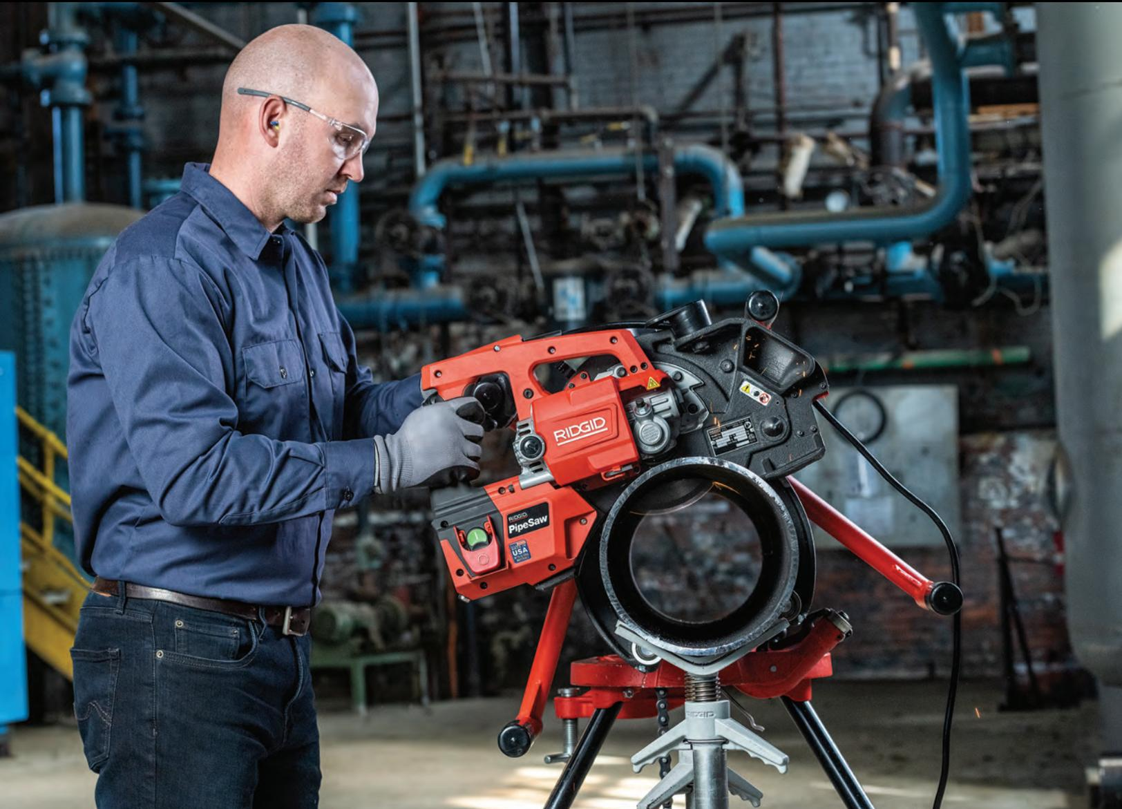
Cut pipe fast and efficiently with the RIDGID® Pipe Saw. From the fab shop to the field, this tool delivers quality cuts on 1" – 12". The tool secures onto the pipe in seconds making setup and operation a breeze. Fast and easy to use, the Pipe Saw lets you focus on the tasks that require more time and effort.
