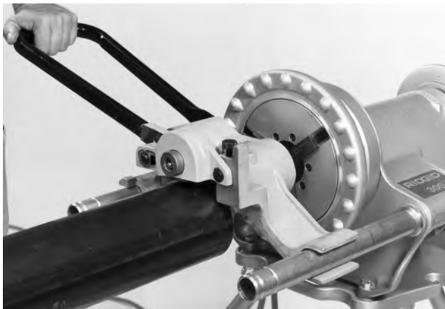
Figure 12 – Forming the Roll Groove
