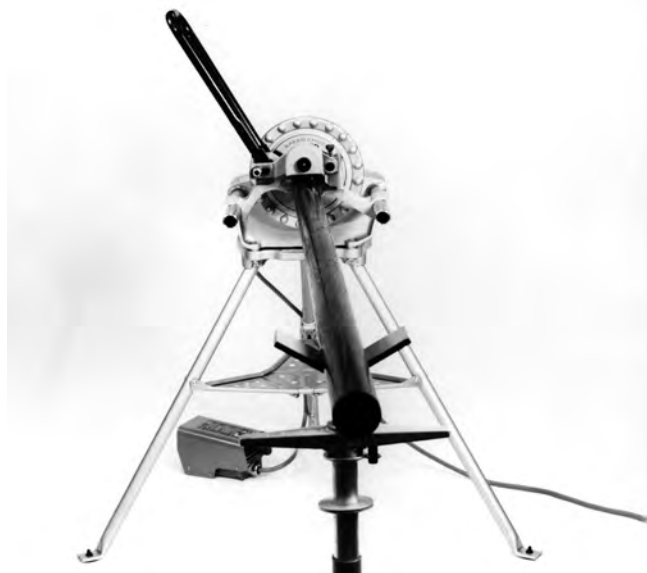
Figure 8B – Operating Machine in FORWARD (FOR) Position
