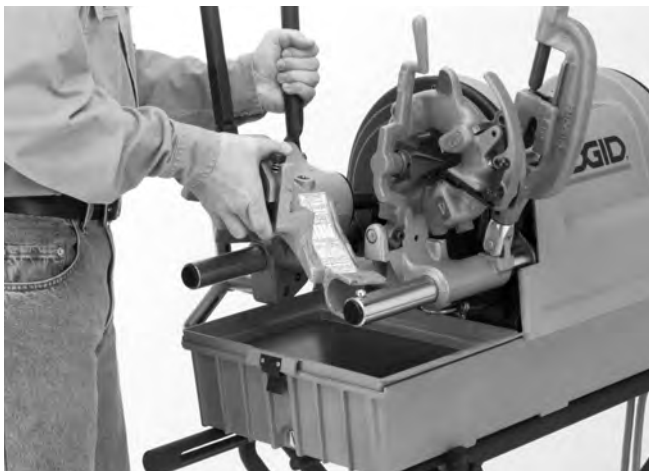
Figure 3 – Mounting on No. 1822-I Threading Machine (Same applies to Models 300 Compact and 535 Threading Machines)
