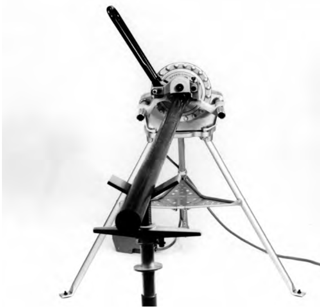
Figure 8A – Operating Machine in REVERSE (REV) Position
