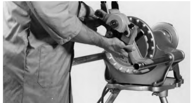
Figure 1 – Mounting on No. 300 Power Drive
