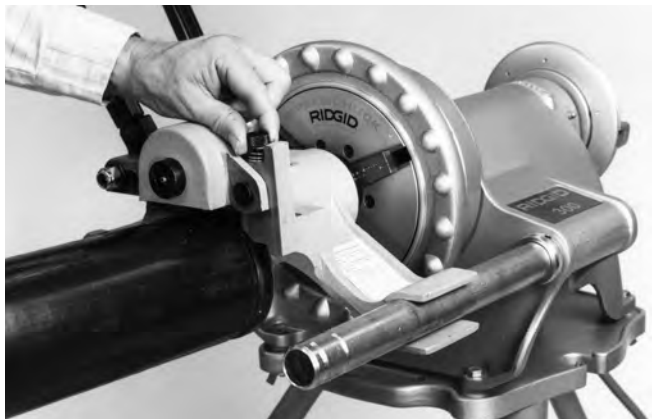
Figure 11 – Tighten Depth Adjustment Screw
