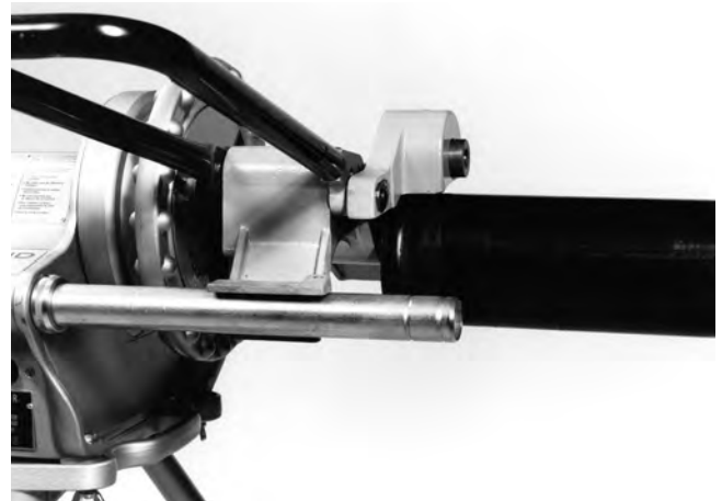
Figure 6 – Square Pipe & Pipe Support
