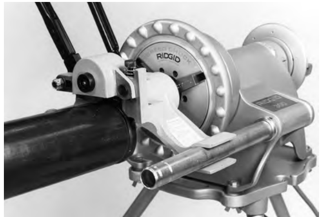
Figure 9 – Feed Handle in UP Position
