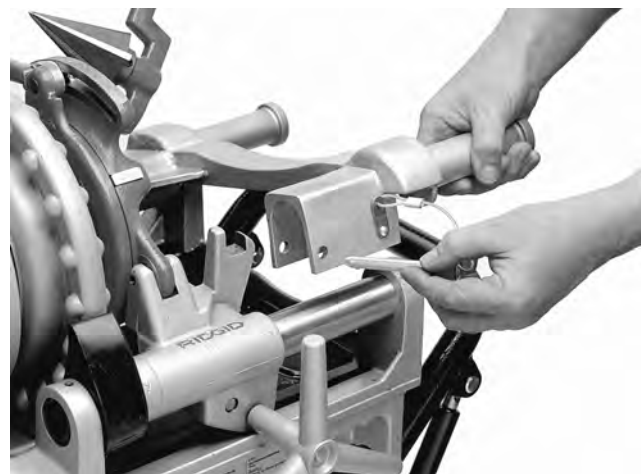
Figure 4 – Attaching Adapter Bracket to 300 Compact Threading Machine
