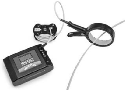
Figure 14 – Inductive Clamp Attached to a Conductor
