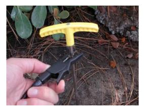
Figure 4: Attaching Lead to Ground Stake
