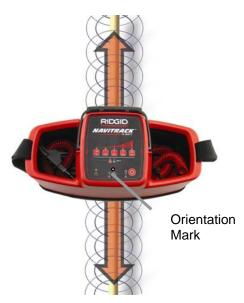
Figure 10: Orientation to Conductor (Inductive Mode)
