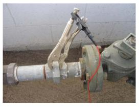
Figure 6: Alternative Connection to a Pipeline
