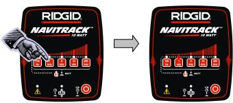
Figure 13: Selecting a 1 kHz Frequency
