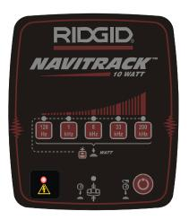
Figure 19: High Voltage Warning LED
