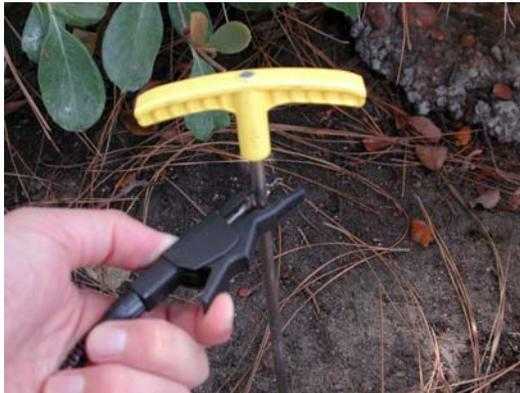
Figure 4: Attaching Lead to Ground Stake
