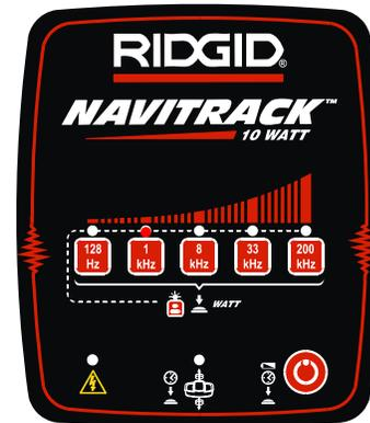
Figure 15: Steady 1kHz LED
