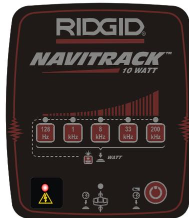
Figure 19: High Voltage Warning LED
