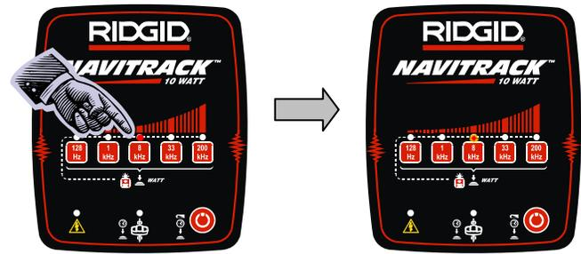
Figure 14: Flashing LED Indicates Medium Power Level
