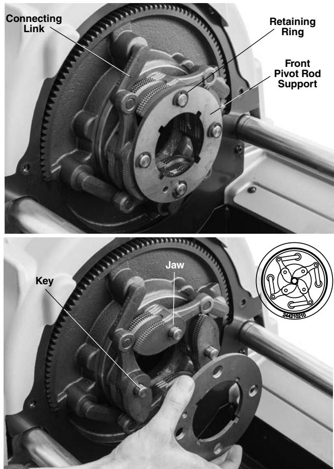
**Figure 32 – Changing Auto Chuck Machine Jaws**
