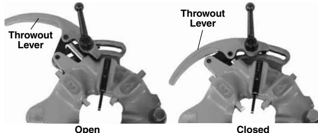
**Figure 9 – Open/Closed Position**
