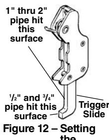
**Figure 12 – Setting the Trigger**
