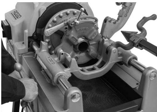
**Figure 23 – Threading Pipe**
