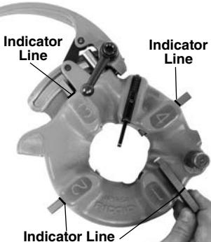
**Figure 10 – Inserting Dies**
