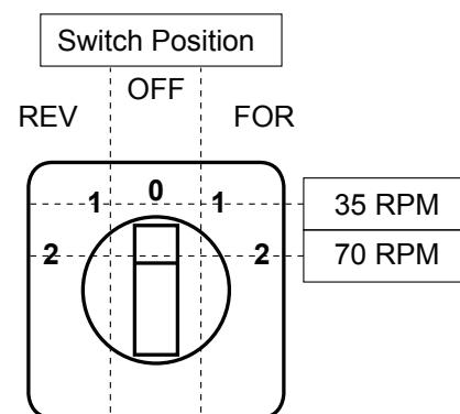
**Figure 19 – 400 V 3 phase Speed and Direction Control**
