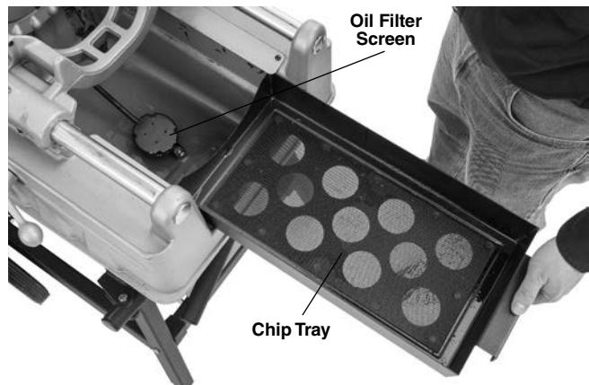
**Figure 30 – Removing Chip Tray**
