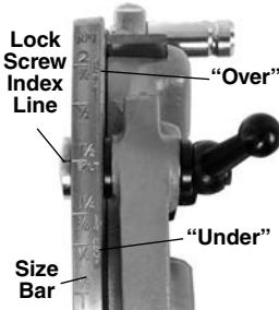
**Figure 11 – Adjusting Thread Size**
