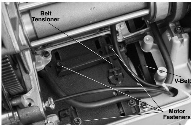
Figure 35 – Belt Tensioning
