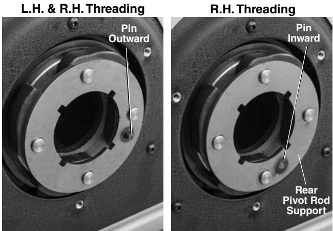
**Figure 25B – Rear Pivot Rod Support - Pin Placement**
