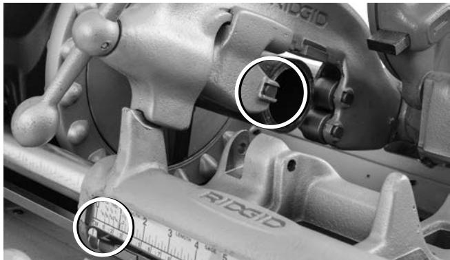
Figure 20A – Cutter Wheel Blade Against End of Pipe. Set Pointer to Zero (0)
