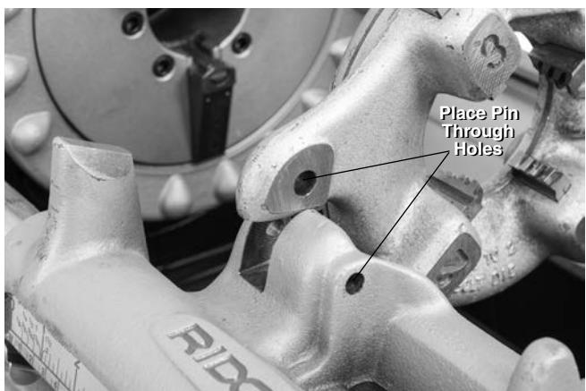
**Figure 26 – Retaining LH Die Head in Place**
