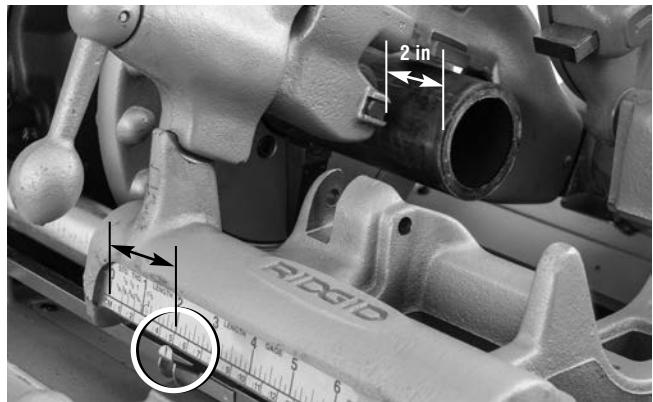
Figure 20B – Length Gauge Pointer At Desired Length
