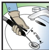
7. Insert cable into the drain opening. At least 12" (30cm) of cable must be in the drain to prevent cable whipping when started. Expose no more than 6" (15cm) of cable between the AUTOFEED unit and drain opening to help prevent cable twisting, kinking or breaking.
