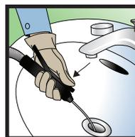
9. To advance the cable into the drain, depress the ADVANCE feed lever on the AUTOFEED unit. If the cable gets stuck in the blockage and stops turning, the drain is not being cleaned. To free the cable from the blockage depress the AUTOFEED RETRIEVE lever.
