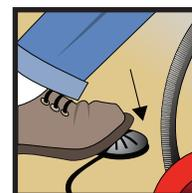
8. Grasping the AUTOFEED unit, move the FOR/OFF/REV switch to the FOR position. Press the foot switch to start the machine.
