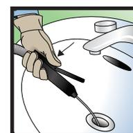
10. Once the blockage has been cleared, depress the AUTOFEED RETRIEVE lever to retrieve the cable from the drain. The FOR/OFF/REV switch should remain in the FOR position. Do not retrieve the cable with the switch in the REV position, this can damage the cable.
