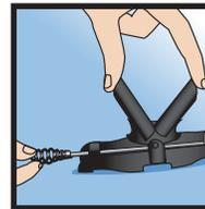
2. Lift the ADVANCE and RETRIEVE levers to allow the bulb head of the cable to feed through the AUTOFEED unit.
