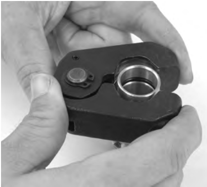
Figure 9 – Installing Press Ring onto Fitting
