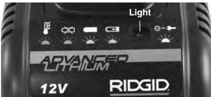
Figure 5 – Charger LED Light and Markings
