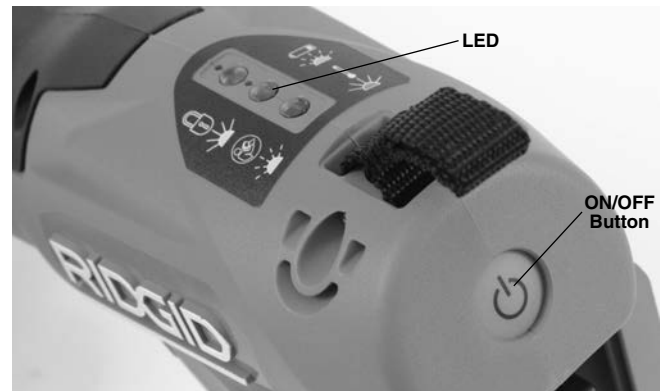
Figure 3 – Tool Status Lights
