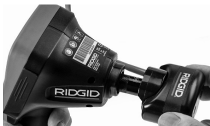
Figur 18 – Kameraets tilkopplingsplugg installert
