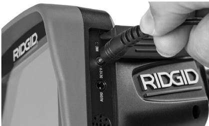
Figure 6 – Powering the Unit with AC Adapter
