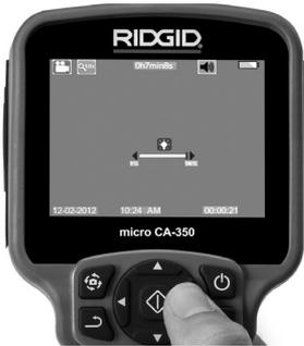
Figure 14 – Adjusting LED
