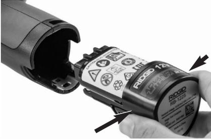
Figure 5 – Removing/Installing Battery
