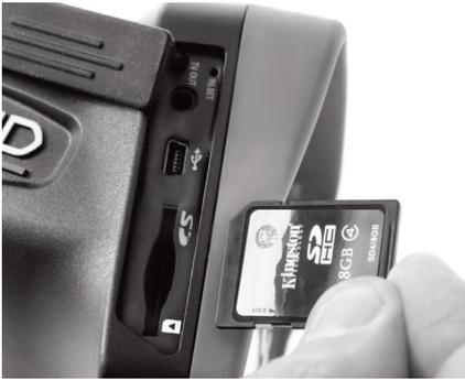
Figure 9 – Inserting the SD Card
