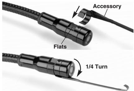
Figure 8 – Installing an Accessory
