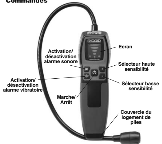
Figure 2 – Composants du micro CD-100
