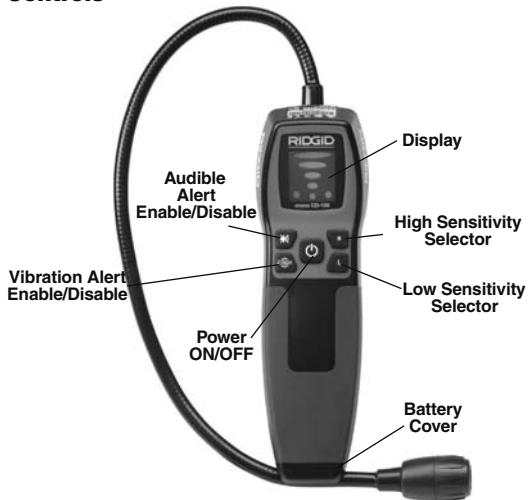
Figure 2 – micro CD-100 Parts
