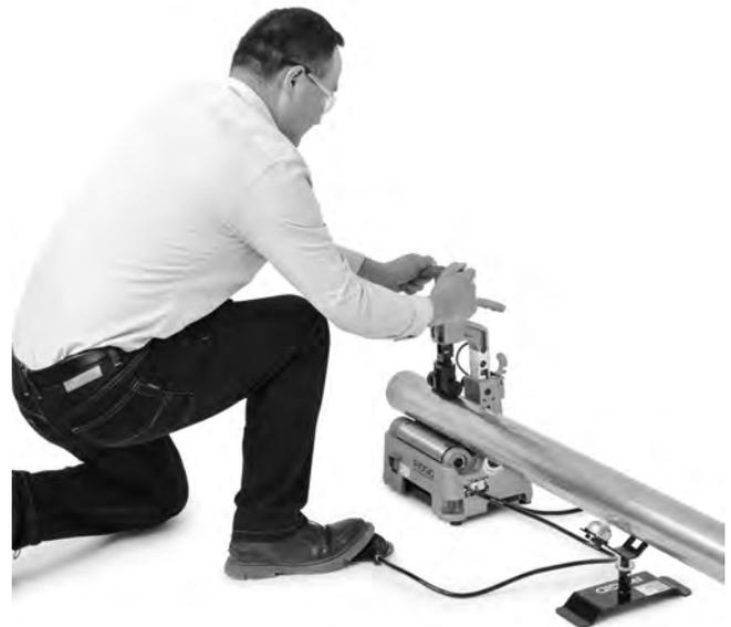
**Figure 10 – Cutting Tubing**
