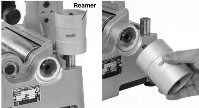
**Figure 11 – Installing Reamer**
