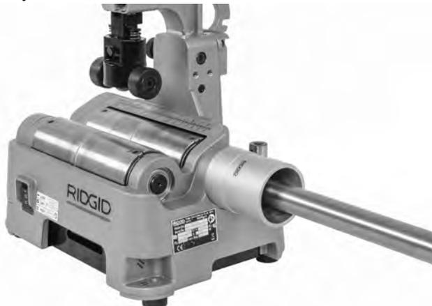
**Figure 12 – Reaming Tubing**
