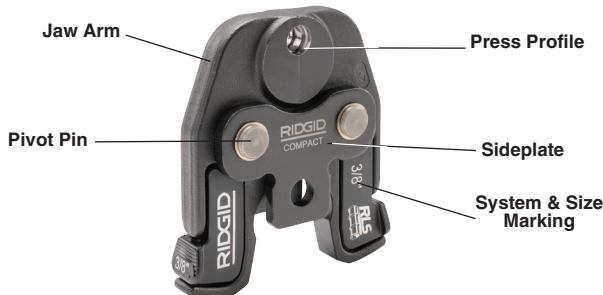
Figure 1 – RLS Refrigeration Press Jaw Set
