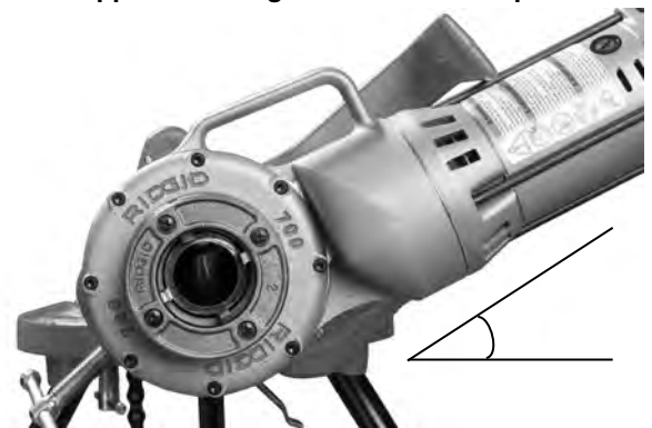
Figure 6 – Support Arm Positioned With 700 Power Drive Slightly Above Horizontal
