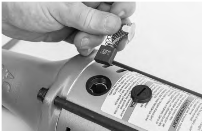
Figure 13 – Installation des balais
