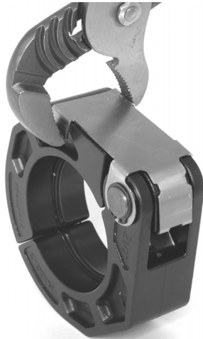
Figure 5 – Using an adjustable pliers to bend the tabs.
