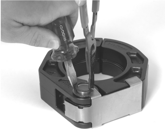
Figure 4 – Installing the retaining rings.
