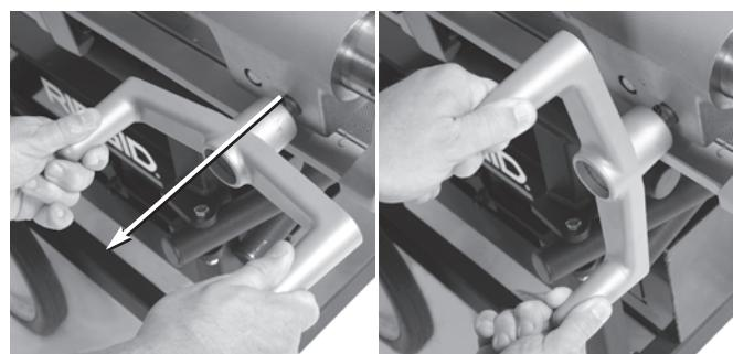
**Figure 20 – Carriage Handwheel Adjustment**
