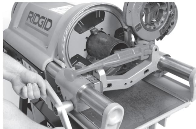
**Figure 22 – Reaming Pipe with Reamer**
