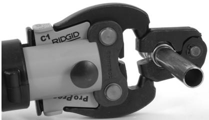
Figure 10 – Attaching Actuator to Press Ring
