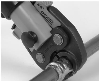
**Figure 7 – Placing Scissor-Style Jaws Around Fitting**
