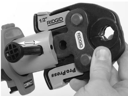
Figure 6 – Attachment Mounting Pin
