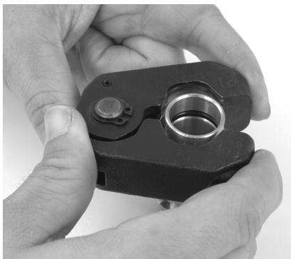
Figure 9 – Installing Press Ring onto Fitting
