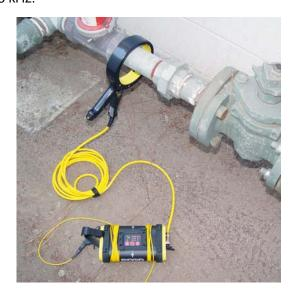
Figure 10: Inductive Clamp Attached to a Conductor
