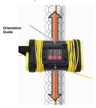
Figure 11: Orientation to the Line – Inductive Mode
