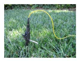
Figure 4: Connecting the ST-305 Ground Stake
