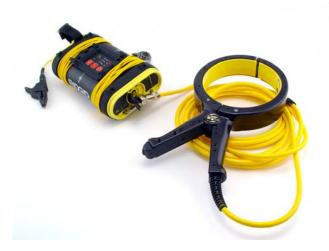
Figure 9: ST-305 with Inductive Clamp
