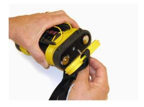
Figure 3: Removing the Battery Cover
