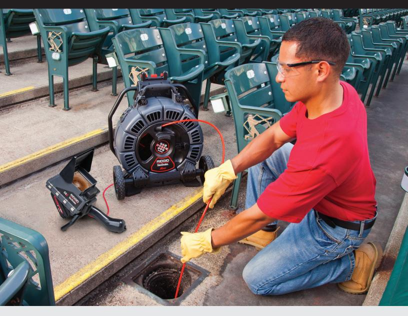
The rM200 Camera System combines portability with the versatility of the D2 drum series, offering different combinations of push cable stiffness and spring flexibility to tackle any inspection job.
