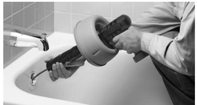
Figure 8 – Keep Distance Between Drain Opening and Nose of Drain Gun to 6" or Less
