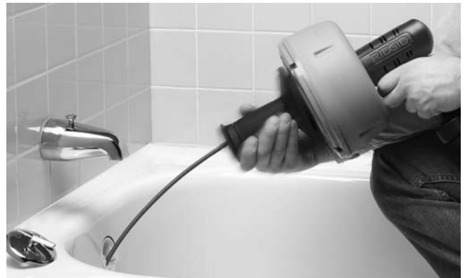
Figure 5 – Pull Hand Grip Rearward To Engage Clutch
