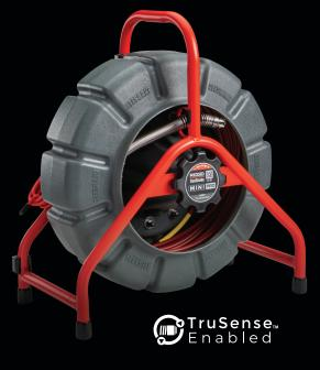
The RIDGID® SeeSnake® Mini Pro™ delivers the most stable in-pipe image with digital self-leveling and TruSense™ Technology. Our shortest 25 mm self-leveling camera head can navigate hard 90° bends while inspecting up to 61 m (200 ft.) with mid-stiff push cable. No moving parts in the camera head greatly enhances the service life expectancy of the camera head.
