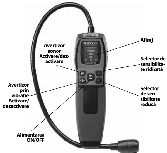
Figura 2 – Componentele micro CD-100
