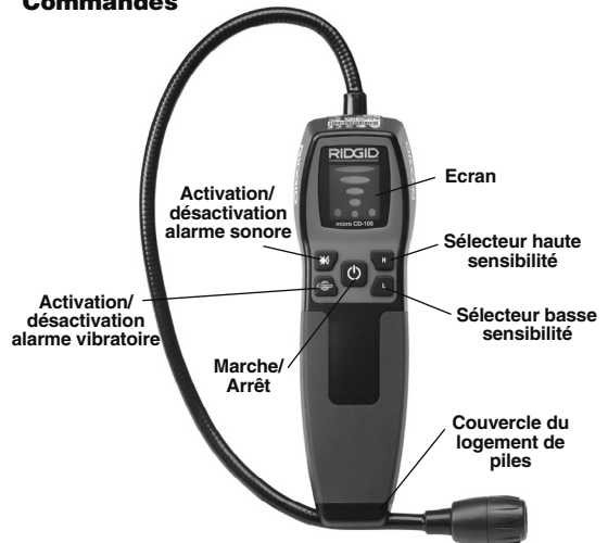
Figure 2 – Composants du micro CD-100
