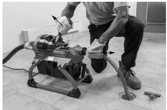
Figure 11B – Clutch released, Cable Not Rotating, Pulling Cable From Machine
