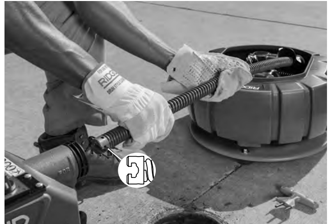
Figure 7 – Inserting Cable Into Front Of Machine
