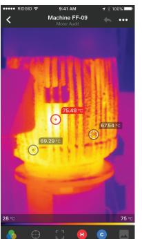
Image Detail screen allows for color palette changes, pinpoint temperature, zoom, high & low temperature and photo mode
