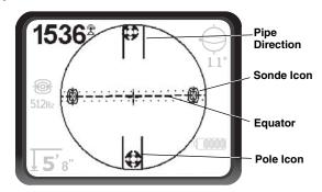
Figure 7 – Display Elements: Sonde Mode
