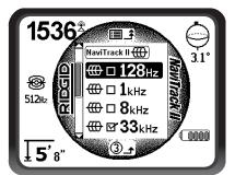
Figure 16 – Highlighting a Desired Frequency (128 Hz)
