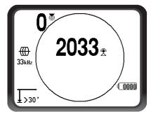
Figure 41 – Signal Strength Centered
