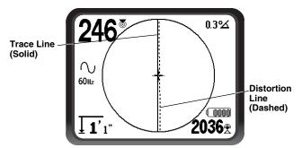
Figure 29 – 60 Hz Passive Trace Frequency
