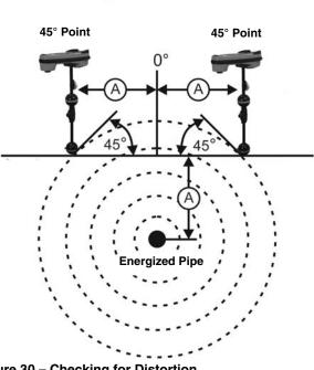
Figure 30 – Checking for Distortion
