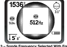
Figure 13 – Sonde Frequency Selected With Frequency Key
