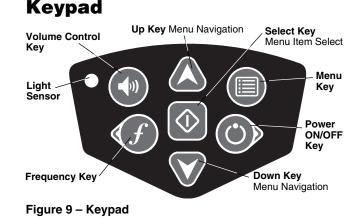
( **Power ON/OFF** – Powers NaviTrack II ON. Powers the NaviTrack II down after a 3-second countdown. The countdown can be interrupted before shutdown by pressing any key.
