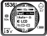
Figure 32 – Selecting Units (Feet/Meters)
