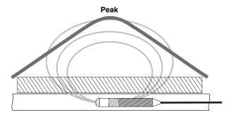
Figure 50 – Sonde signal as "seen" by the NaviTrack II The only way to go is "up" toward the maximum signal.
