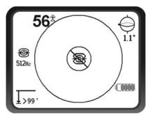
Figure 40 – "No-Signal" Display in Sonde Mode
