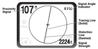
Figure 8 – Display Elements (Line Trace Mode)
