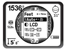
Figure 33 – Setting Backlight Mode (On/Off/Auto)
