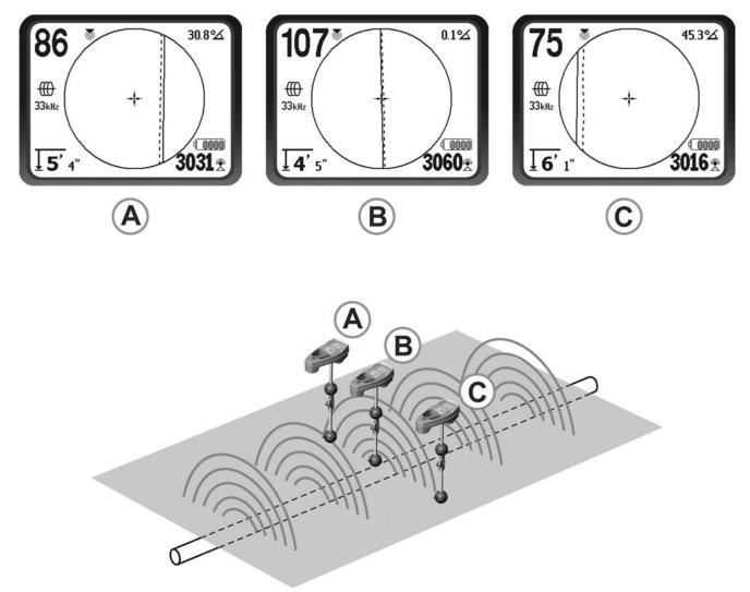
Figure 28 – Screen Display in Different Locations (Active Line Tracing)
