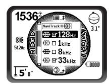
Figure 18 – Desired Frequency Checked
