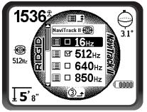
Figure 43 – Highlighting a Frequency to Activate
