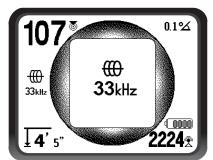
Figure 26 – Line Trace Frequency Chosen with the Frequency Key
