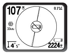
Figure 10 – Display Low-Battery Warning
