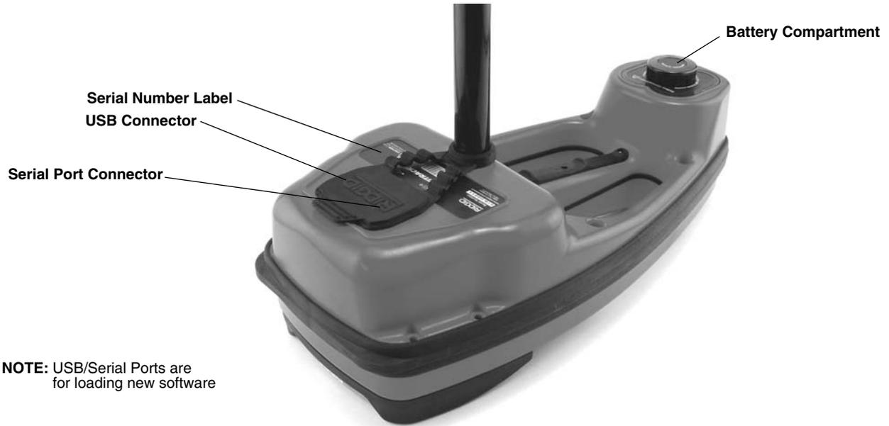
**NOTE:** USB/Serial Ports are for loading new software
