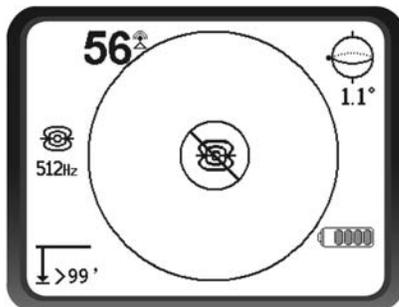
Figure 40 – "No-Signal" Display in Sonde Mode
