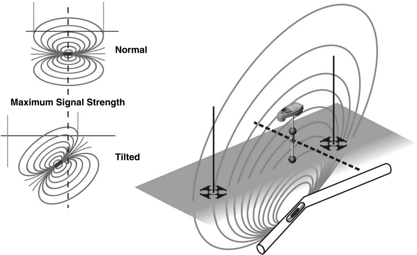
**Figure 25 – Tilted Sonde, Poles and Equator**
