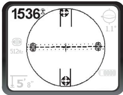
**Figure 23 – Sonde Locate: Equator**
