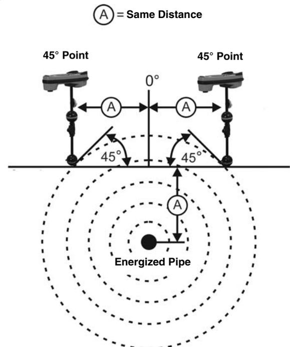
**Figure 30 – Checking for Distortion**
