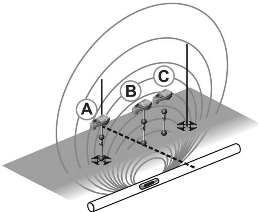
Figure 24 – Screen Display in Different Locations (Sonde)
