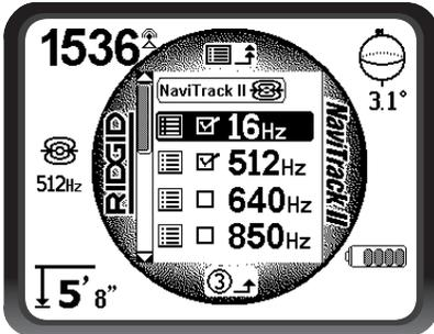
**Figure 44 – Selecting a Frequency to Activate**
