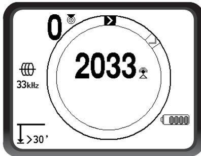
Figure 39 – Racetrack with Watermark and Pointer
