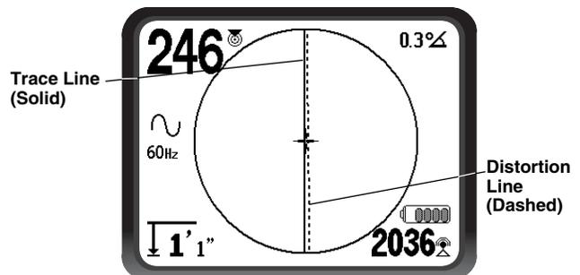
Figure 29 – 60 Hz Passive Trace Frequency
