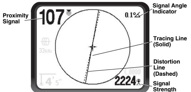
**Figure 8 – Display Elements (Line Trace Mode)**
