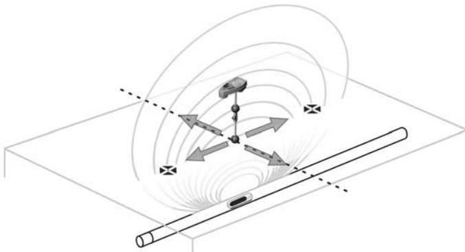
Figure 22 – Poles and Equator of a Sonde
