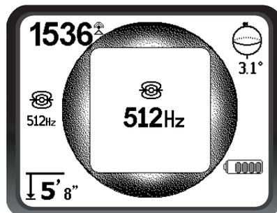
**Figure 13 – Sonde Frequency Selected With Frequency Key**
