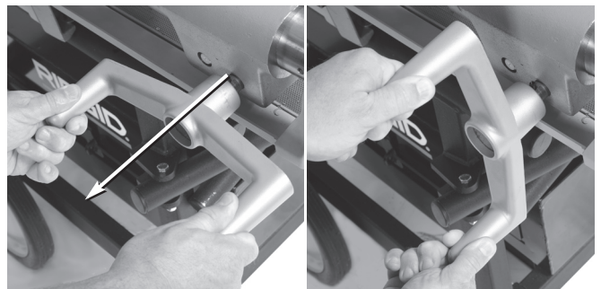
Figure 20 – Carriage Handwheel Adjustment
