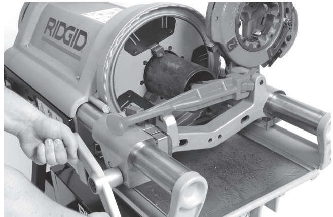
Figure 22 – Reaming Pipe with Reamer
