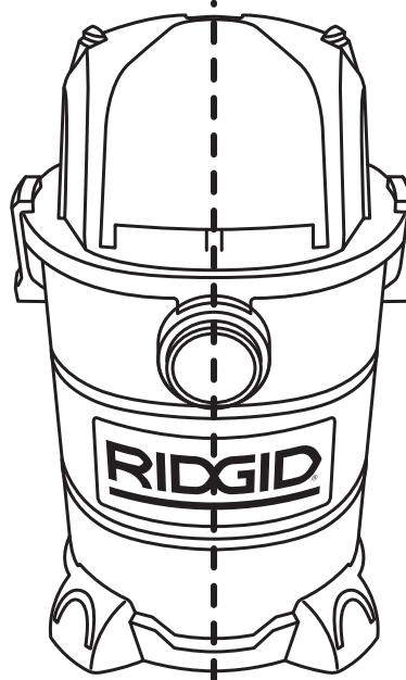
Next, secure the caddy between your feet to hold it in place. Grasp the upper rim of the drum and rotate until the inlet is centered between the caster feet of the caddy.
