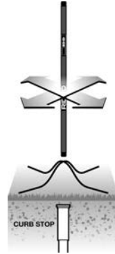
Figure 9 – Specific Locate Signal
